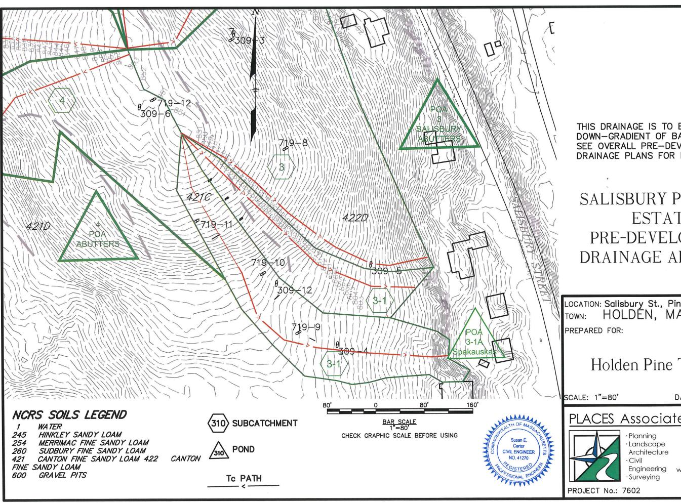
THIS DRAINAGE IS TO EXAMINE DRAINAGE DOWN-GRADIENT OF BASIN D-3 ONLY. SEE OVERALL PRE-DEVELOPMENT DRAINAGE PLANS FOR REMAINING AREAS.
